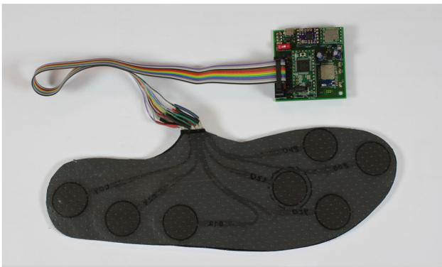
**Fig. 6** Preview of a single insole with its microcontroller of the SONIGait 2.0 device. For a better visibility of the sensor placement and associated wiring the top layer of the insole is illustrated transparently. Utilizing the A401 model will increase the sensing area per force sensor from 0.71 to 5.07 cm<sup>2</sup>
