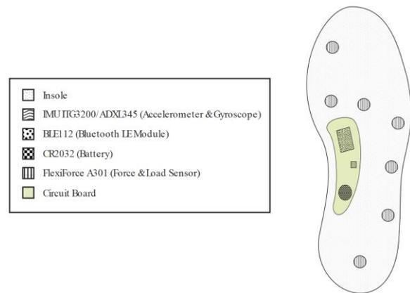
Figure 6: Desired form factor for the SONIGait device for future iterations in development.
